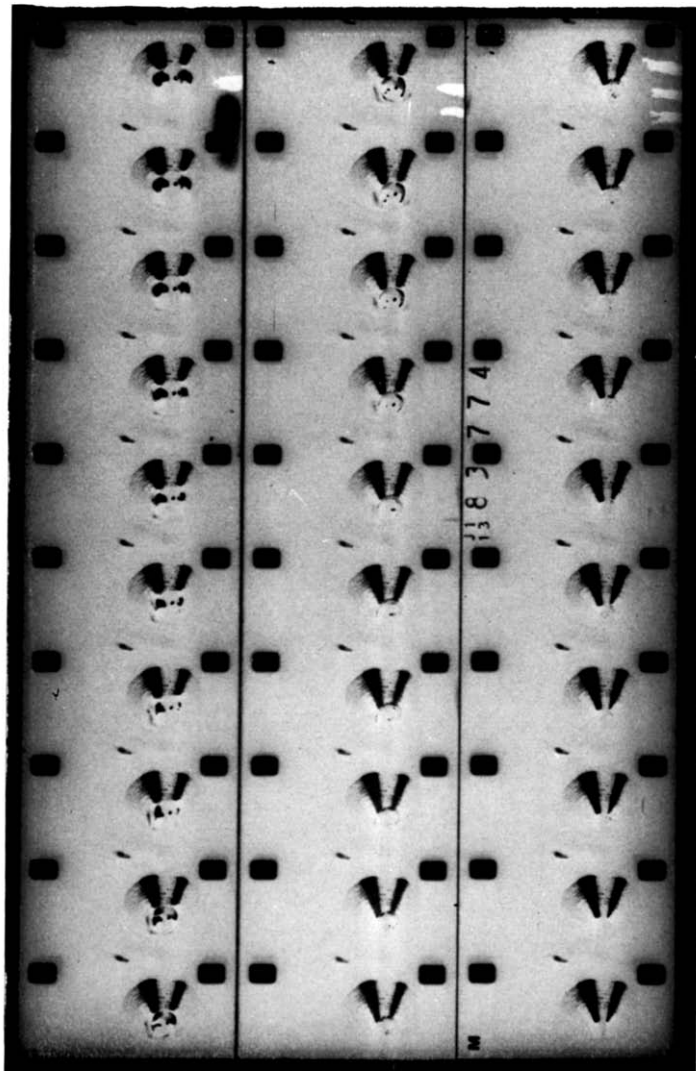
FIG. 8. Negative print of high-speed moving picture of drop interacting with heat-transfer surface (specimen 1). Frame rate is 3700 frames per second. Water drops; d = 3.89 mm, D = 3.53 mm, f = 300 drops per min, T_s = 550^\circ\text{K} .
